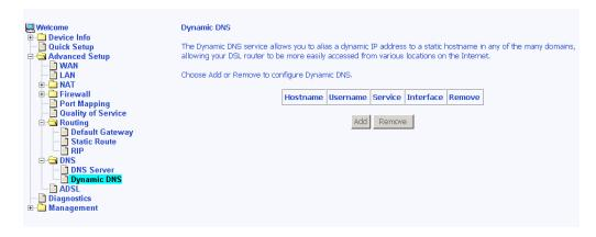
This screen allows you to add a dynamic DNS address from DynDNS.org or TZO. Enter the hostname and the interface that you are using. Also enter the username and password assigned by the DNS service. Click on **Save / Apply** to save these configurations.
